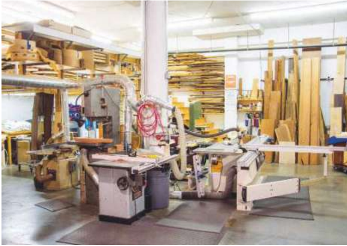
Craig's workshop, where most of his tools are located. "I have a variety of power tools including an 8ft sliding table saw, 254mm Unisaw, 508mm bandsaw, 406mm bandsaw, 100mm edge sander, 2ft curved edge sander, 330mm planer and a 203mm jointer". There's also a 3hp cyclone dust collector on the left just out of camera shot, plus a drawing area and vacuum table shown on the left
